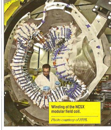
between Mylar and Kapton tape. Both provide needed electrical isolation. But Kapton, a polyimide film, better withstands cryogenic temperatures during NCSX operation without turning brittle or losing critical properties. Temperature was also a factor in selecting epoxy. It must hold up under liquid-nitrogen operating temperatures without cracking.
