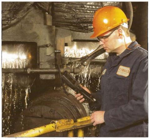
An engineer checks a machine with a handheld vibration analyzer.
