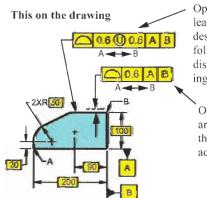
Option 1: The profile tolerance is a total of 0.6. The leader arrow points directly to the surface. The circle U designates the tolerance is an unequal tolerance. The 0.6 following the circle U designates the tolerance zone is displaced by 0.6 to the outside of the true profile indicating the direction that adds material.
