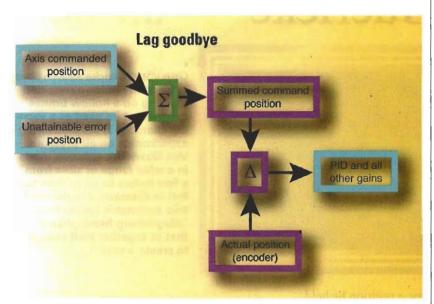
Triggered gear move command sets allow an axis to accelerate to a master encoder in a fixed length of product, despite encoder speed variances. Triggered *cam* commands make cams start on a trigger and accelerate to geared line speed — despite varying line speed — to accelerate the cam to line speed over a fixed, known length.
