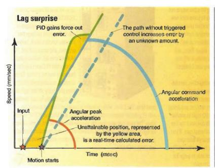
When a trigger input is fired, a signal tells the system to move — red star. At first, because of unavoidable servo lag, the system does nothing. Then, the system starts to move — purple star. But it's different than the motion we might expect see — light blue dashed line.
