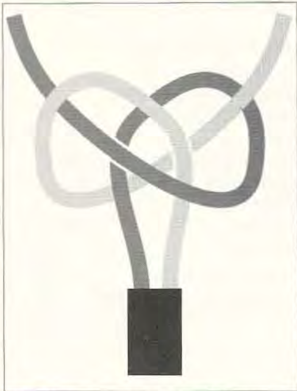
Fig. 3. The "Electrician's" or "Underwriter's" knot.
