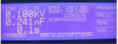
If measured  $C_m$  is > 0.121nF the result is Pass,
