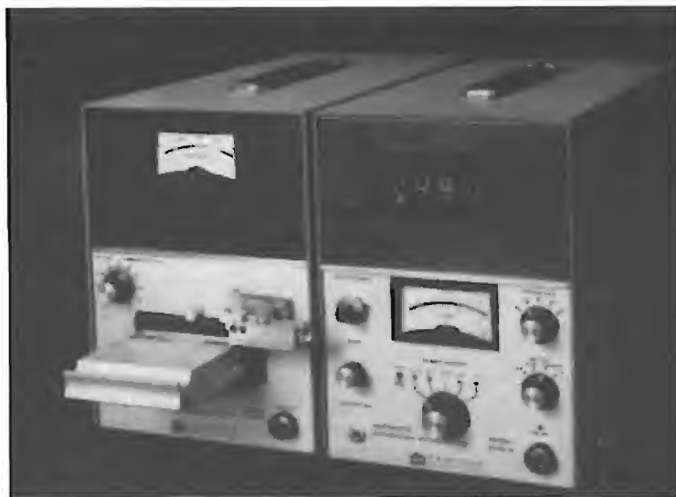
A complete thermoluminescence analyzer. Unit at left contains sample drawer, heater, and photomultiplier; the unit at the right contains the integrator and the digital readout.
