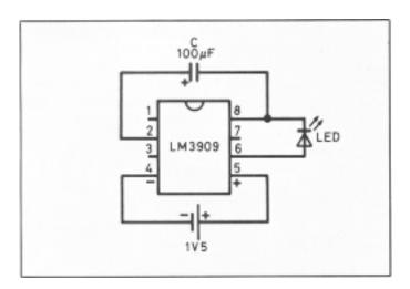
Figure 1 Circuit diagram of the LED Flasher. Pins 1, 3 and 7 of the IC are not used
