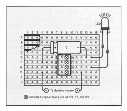
Figure 2 Board layout viewed from the component side. The tracks are cut under the board where shown
