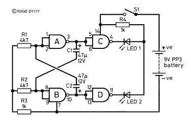
Figure 1 Flashing LEDs, circuit diagram
