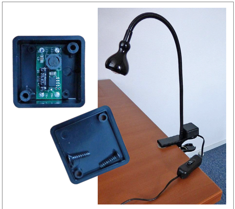
Figure 4. The author has put his prototype in a small Hammond enclosure, which was then fixed onto the clamp of the spotlight.
