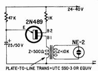
low-power pilot-lamp circuit for transistorized equipment operating from 24-40-volt batteries. Power drain is reduced by using a flashing indicator
