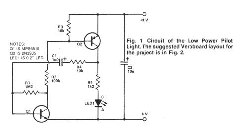
struction techniques: either Veroboard or PCB can be used to build it up. Overlay and connection details are given for them both in Figs. 2 and 3.
