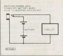
Fig. 2. Using a battery eliminator.
