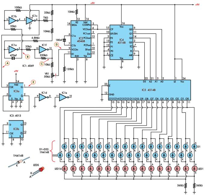
the 180nF capacitor between pins 6 and 7 and by the control voltage fed to it at pin 9, ie, the  $\sim$ 0.5Hz sinewave.
