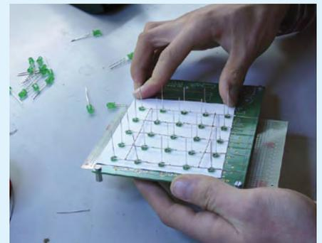
of the 25 column leads over by about 3 mm, to reach around the LEDs of the previous layer. The second layer is subsequently placed above the first layer and we solder this layer at every connection, with a uniform spacing between the layers and the LEDs neatly lined up.
