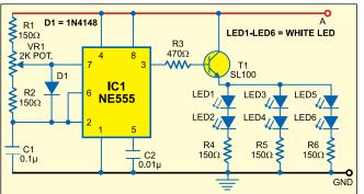
Fig. 1: White LED based emergency lamp
