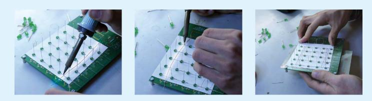
of the 25 column leads over by about 3 mm, to reach around the LEDs of the previous layer. The second layer is subsequently placed above the first layer and we solder this layer at every connection, with a uniform spacing between the layers and the LEDs neatly lined up.
