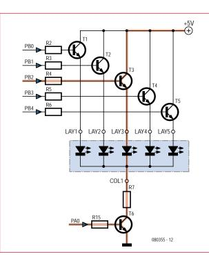
Figure 2. In this figure you can see the path that the current takes through the middle LED in the first column.
