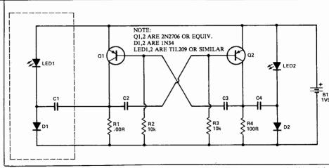
alternately, C1 and C2 should be about 1000uF. To operate only one LED omit the circuitry within the dotted box.
