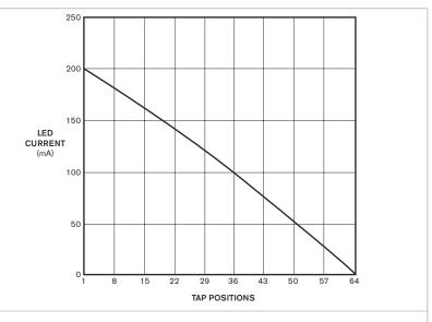
Figure 2 A plot of LED current versus tap position in Figure 1 exhibits only a slight nonlinearity.
