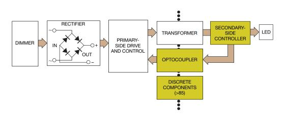
Figure 1 The feedback circuit in a typical offline LED driver circuit requires secondary-side regulation via an optocoupler and many discrete components, resulting in a large bill of materials and a lower overall lifetime for the LED driver.
