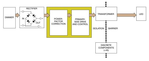
Figure 2 PrimAccurate primary-side digital control architecture reduces the LED driver circuit's external component count and eliminates the need for an optocoupler, thereby improving solid-state-lighting bulb reliability.
