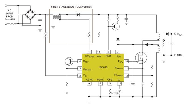
Figure 3 The circuit in this example of a two-stage, high-power-factor-correction LED driver (the iW3616) uses an NTC resistor to provide LED overtemperature protection and derating, thus extending bulb lifetime.
