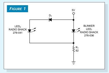
This blinking-LED circuit, designed by a seventh grader, uses only four parts.
