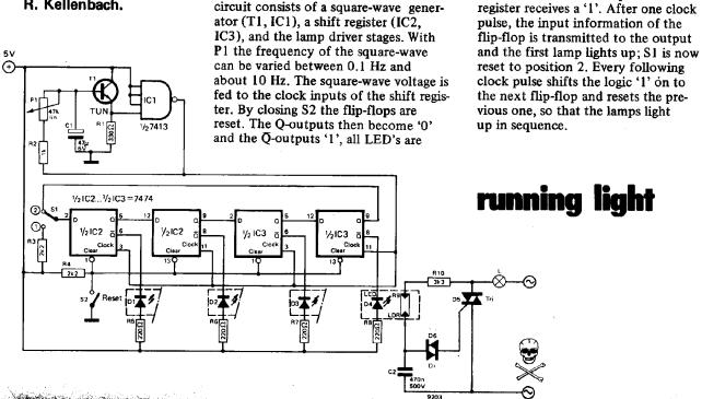
By means of this circuit four lamps can
