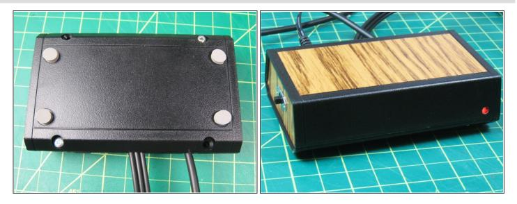
• After confirming that the circuit works, screw the case closed, add rubber feet, and put on any finishing fake wood touches. Attention to detail is proportional to the amount of marvel in your friends' eyes the first time they see your Pixelmusic 3000 in action.
