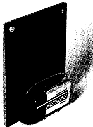
FIG. 7—THE 9-VOLT BATTERY and battery clip act as a stand.
