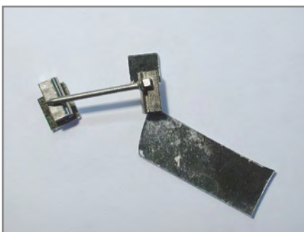
A small nail holds the magnet in place for gluing.
