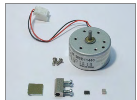
All parts of the servos together: mirror, shaft coupling, magnet sensor and the little magnet.
