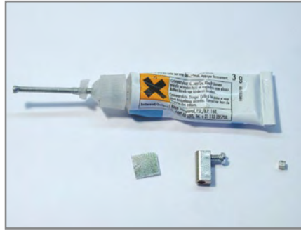
The mirror, the shaft coupling and the little magnet, ready to be glued together.
