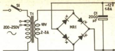
Fig. 1.5. Power supply circuit for the colour display
