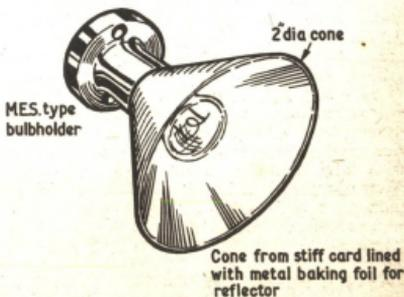
Fig. 1.3. Lampholder and reflector
