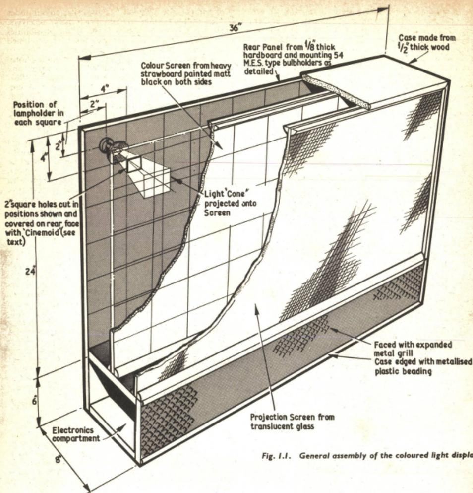
Fig. 1.1. General assembly of the coloured light display
