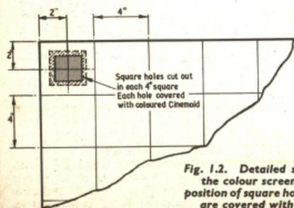
Fig. 1.2. Detailed section of the colour screen showing position of square holes which are covered with coloured "Cinemoid"
