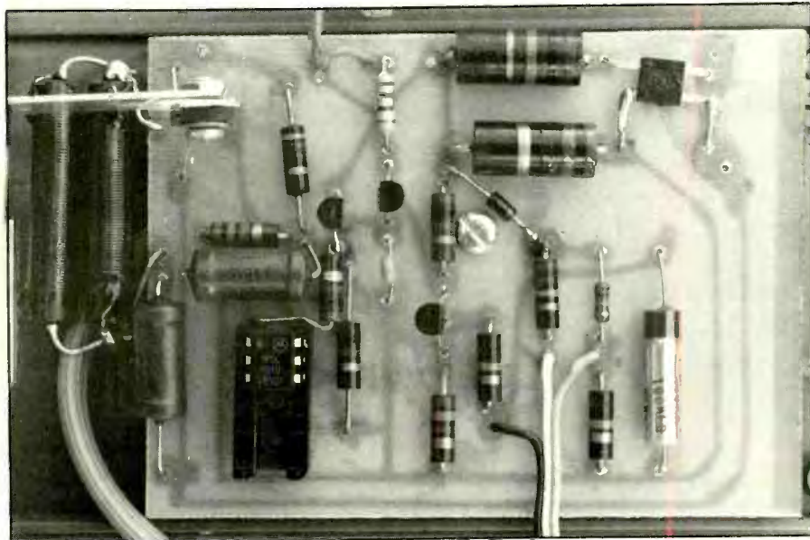
Fig. 3. Note in this close-up view how two chokes are wired in parallel for L1 and the L-bracket heat sink used for Q4 (upper-left), use of a 16-pin socket for IC1 (lower-left), and single screw that mounts the board on the box (center).
