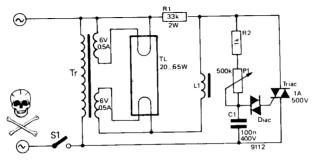
The luminous intensity of fluorescent lamps cannot be controlled by means of conventional light dimmers, unless certain modifications are carried out. In the circuit described here the heaters of the fluorescent lamp are pre-heated by means of a heater transformer with two separate windings. The starter is
