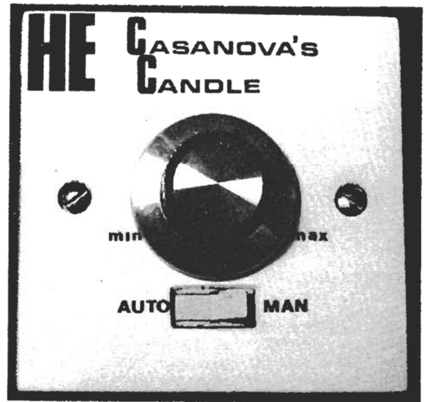
The type of switch used is unimportant, it must, however be of the double pole changeover type.
