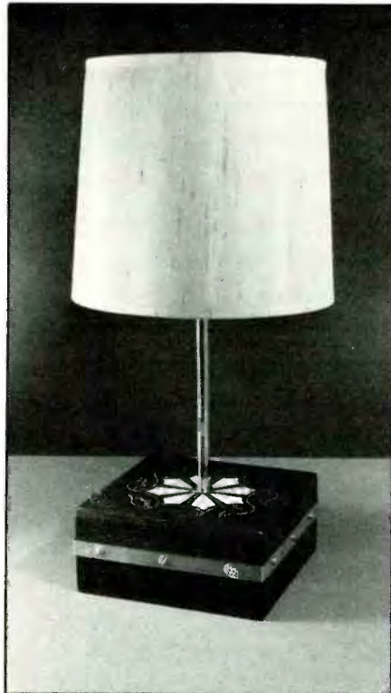
This simple 3-way lamp is controlled by the touch of a finger on the brass band of the wooden base that contains the Touchmaster module.
