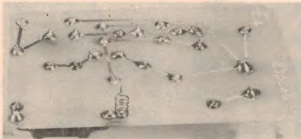
View of the assembled remote control circuit. Note the spring used to provide the contact between the PCB and the metal touch plate.
