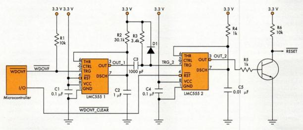
1. The first LMC555 detects the watchdog-overflow trigger from the microcontroller and provides a delay. The second LMC555 allows the firmware to disable the impending hardware reset.
