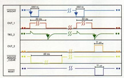
2. This timing diagram for two separate watchdog events shows the reset pulse being held off and not resetting the hardware for the first event and then a reset pulse that occurs after a pre-determined delay for the second event.
