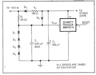
**Resets if necessary.** During brief interruptions of dc power, the charge on  $C_2$  maintains voltage to C-MOS digital circuits, preserving their logic states. But if the power failure lasts so long that the voltage across  $C_2$  drops below 3 V, the Schmitt trigger resets the logic circuits when power is restored.
