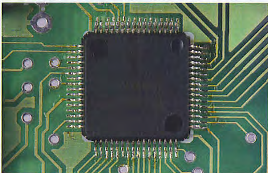
Figure 6. Tiny and tricky to solder: the USB microcontroller comes in a 64-lead SPFP package.
