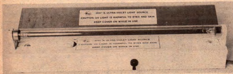
TOP & BELOW: These three views show the UV light source at various stages of assembly. Devices to be erased are placed under the tube for 30 minutes.
