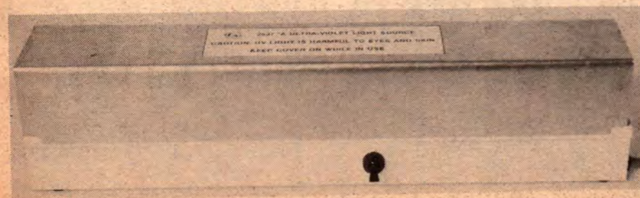
The ends of the top cover are bent so that it sits naturally on the batten.
