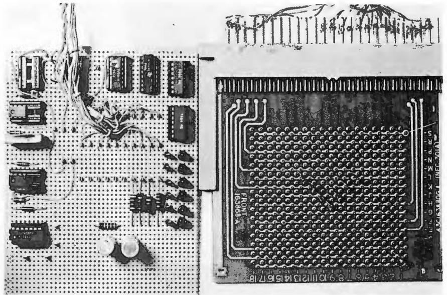
Photo shows the author's prototype of complete PLA project. Diodes are on commercial matrix board at right. IC's and other electronics are on perf board.
