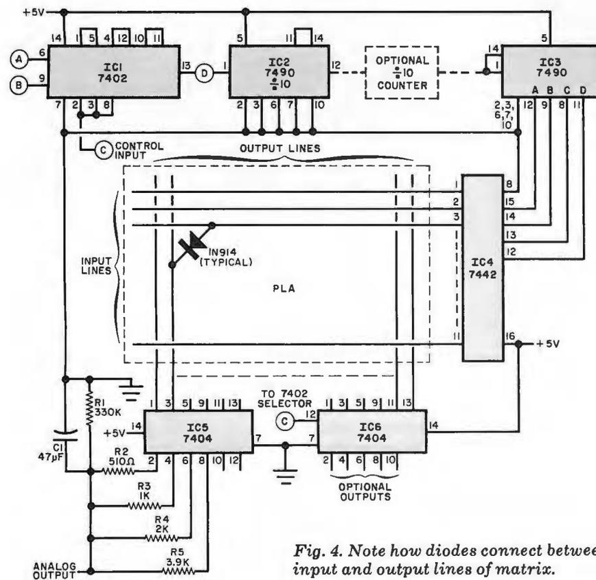
Fig. 4. Note how diodes connect between input and output lines of matrix.
