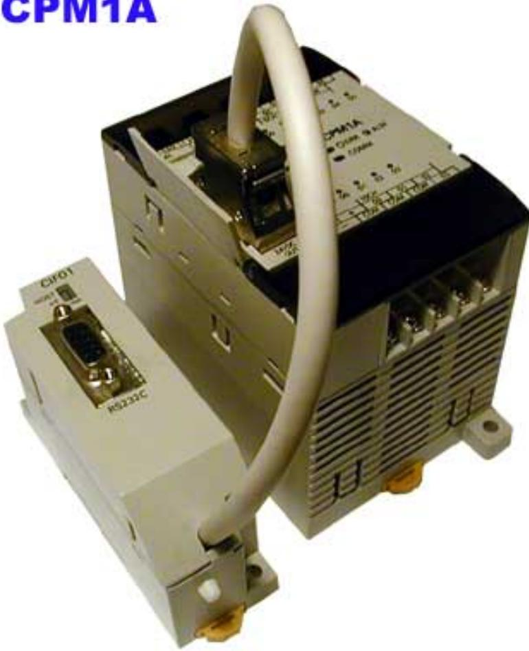
To better inform programmers on PLC controller status, maker has provided for four light indicators in the form of LED's. Beside these indicators, there are status indicators for each individual input and output. These LED's are found by the screw terminals and with their status are showing input or output state. If input/output is active, diode is lit and vice versa.
