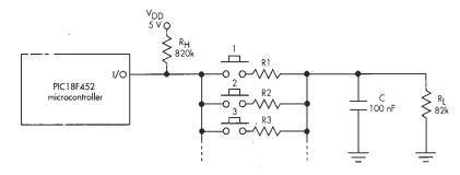
This keypad interface technique controls multiple keys using only one (bidirectional) pin on the microcontroller and a minimum of external components.
