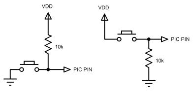
' Goto notpressed if button not pressed on Pin2 BUTTON PORTB.2,0,100,10,B2,0,notpressed
