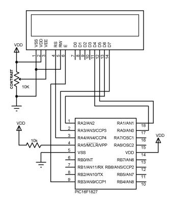
Note that most of the pins used to connect the LCD in the above diagram have the additional function of analog conversion inputs on the 16F1827 (AN0-AN4, and AN9). For proper operation of the LCDOUT command, these pins must be configured as digital I/O with following register settings in the program code:
