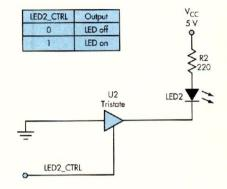
2. If the blinking function isn't needed, the LED control circuit can be simplified as shown.
