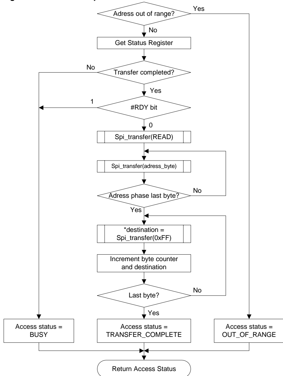
Figure 3-5. GetCharArray flowchart
