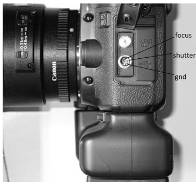
Figure 4-5 Canon 40D shutter-control connector.
