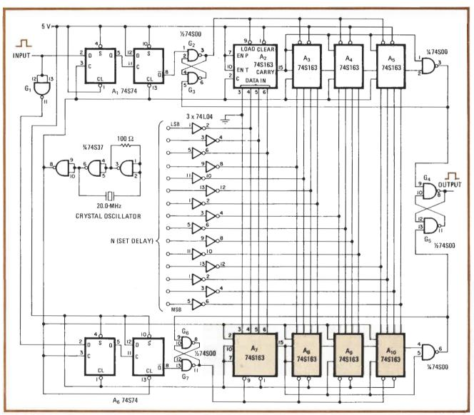
**Two-edge retardation.** Counter chains, of which one starts counting on arrival of the positive edge of an input pulse, the other on its negative edge, use a 20-MHz clock to provide repeatable delays of 50 ns to 3.25 ms on both edges of signal. Delays produced are accurate to within 50 ns. Amount of delay is selected with 15-bit word (M). Width of input signal to be processed must be at least 60 ns.
