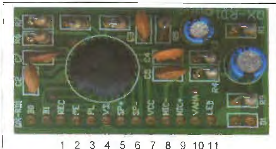
Figure 1. QX series sound recording module. Overall size 45mm x 24mm x 5mm. Pin connector pitch: 0.1 inch. The above module is 20 second 4 segment version. You can use B0 and B1 to select the start of a segment.
