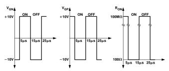
Figure 10. Timing used for simulation in Figure 11.
