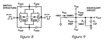
Figure 8. CMOS Switch Structure showing parasitic capacitance. Figure 9. Equivalent circuit showing the main parasitics which contribute to charge injection.
