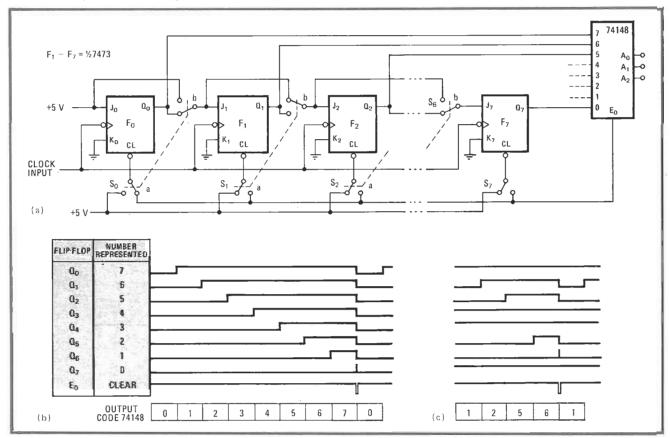
**Chosen order.** Periodic-sequence generator (a) produces selectable, monotonically increasing binary output code (b) having zero dead time. Any number can be omitted from the sequence (c) by using double-pole, double-throw switches to disconnect Q output of the flip-flop corresponding to that number from succeeding flip-flop and bringing its clear port to 5 V.
