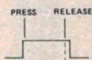
Figure 14. "Debouncing" a press button switch. Such circuits are widely used in logic applications.
