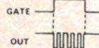
Figure 11. A variation on the circuit in Figure 10 allowing gated operation of the multivibrator.
