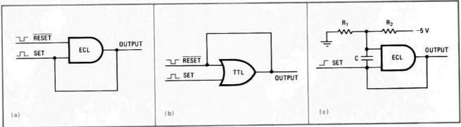
Getting a bistable from a gate. Wired-OR connection (a) from the output of an ECL AND gate to one of its inputs permits the gate to function as a flip-flop. For a positive SET pulse, the output is high; for a negative RESET pulse, the output is low. Similarly, a TTL OR gate (b) with a wired-AND connection to one of its inputs also acts as a flip-flop. A simple RC network (c) can be added to produce a one-shot.
