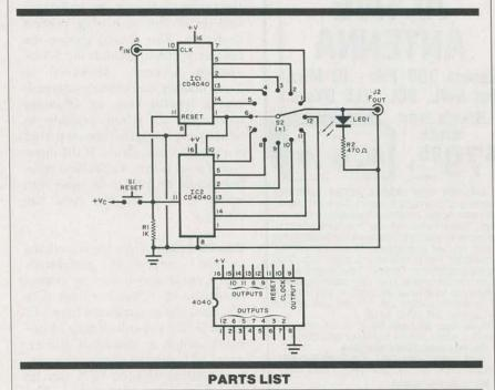
IC1,IC2—CD4040 12-stage counter LED1—Any light-emitting diode J1,J2—Miniature open-circuit phone jack R1—1-kilohm, ¼-W resistor
