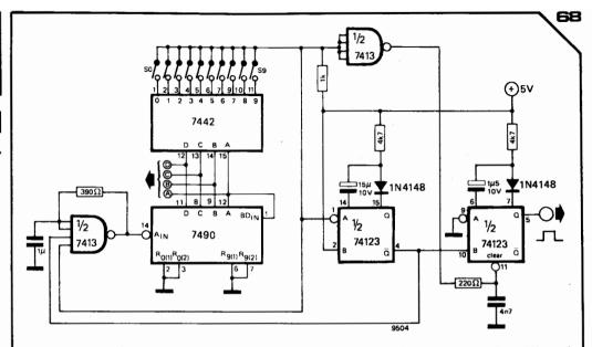
When one of the keys S0...S9 is pressed the keyboard decoder generates the BCD code which corresponds to that key. To ensure that only the desired BCD information is read out the circuit also produces a strobe pulse which indicates that the information has been accessed.
